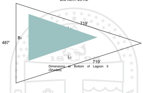
Slope is 3:1 (3 feet horizontal for every 1 foot height) Top dimensions at elevation 575.6.
