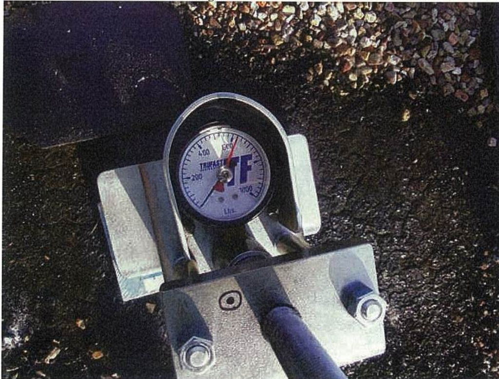
Photo #4 View of fastener pull test at Bldg. B006. Failure at 610 lbs force.
