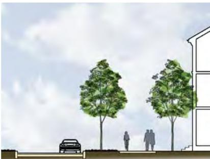
*Section through a trail-width sidewalk. Sidewalk, verge, and setback are 10 feet each, allowing for ample biking and walking space.*
