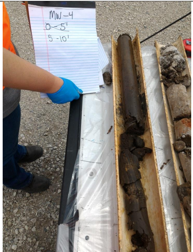
Close-up view of the core recovered from MW4 – 5-10'
