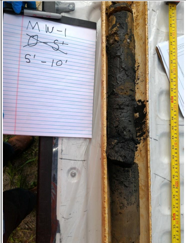
Close-up view of the core recovered from MW1 – 5-10'
