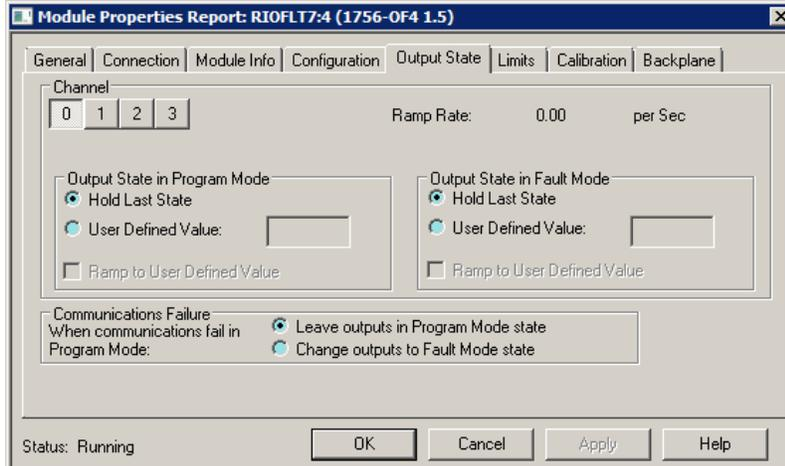
**Figure 5-5 PLC Analog Output Card Output State Configuration**
