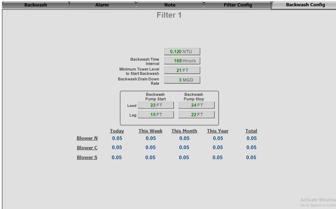
Figure 6-51 Filter Control Popup Backwash Config Tab
