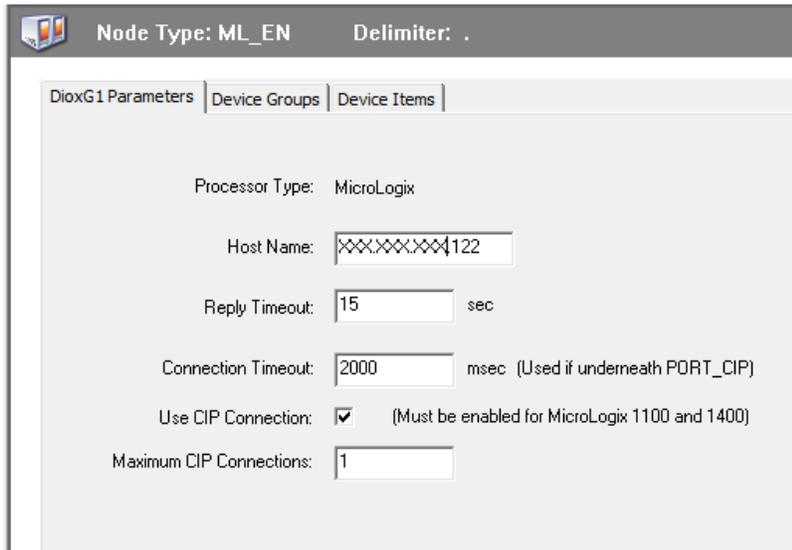
**Figure 6-7 SMC Micrologix Configuration**
