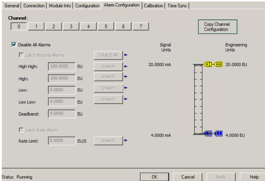
**Figure 5-3 PLC Analog Input Card Alarm Configuration**
