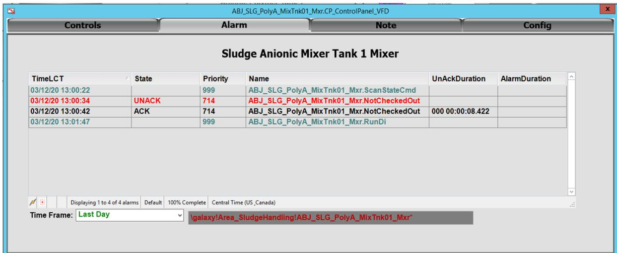
Figure 6-54 \$ComplexMotors Template Popup Alarm Tab
