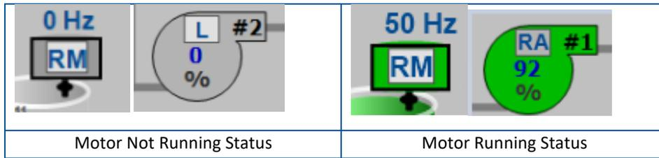
Figure 6-52 \$ComplexMotors Template Graphic
