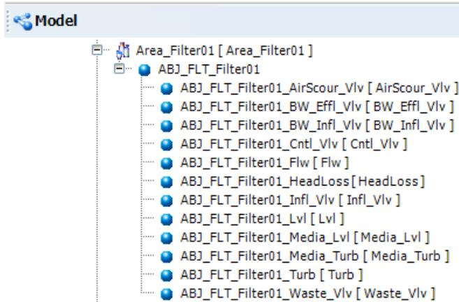
**Figure 6-12 Filter Containment**
