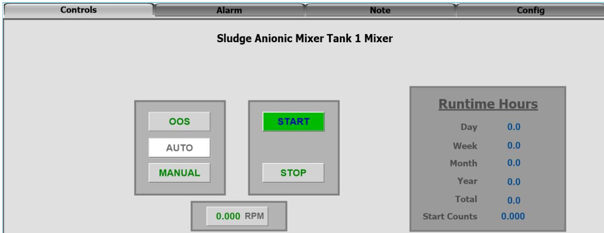
Figure 6-53 \$ComplexMotors Template Popup Controls Tab
