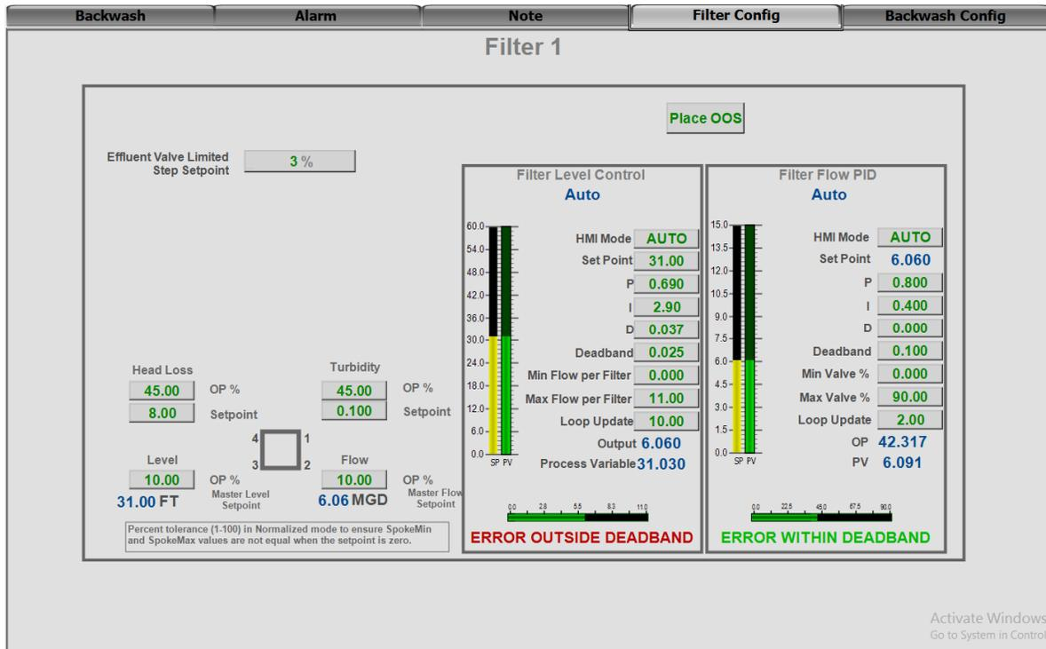
Figure 6-50 Filter Control Popup Filter Config Tab
