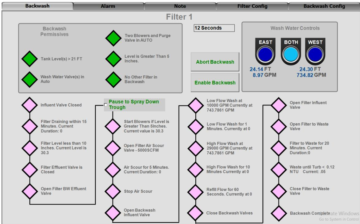
Figure 6-47 Filter Control Popup Backwash Tab
