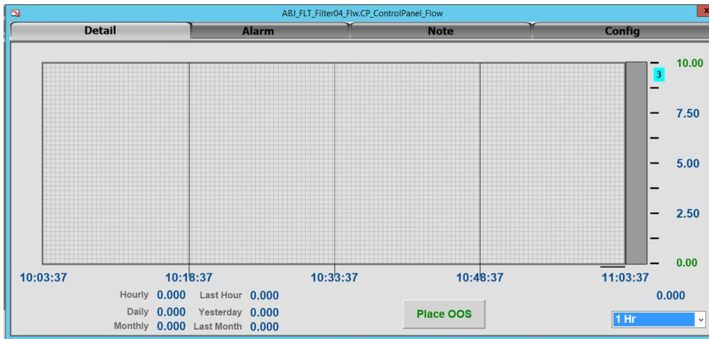
Figure 6-36 Analog Flow Value Popup Detail Tab
