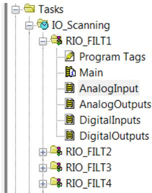
Figure 5-1 Signal Addressing Routine Structure in PLC
