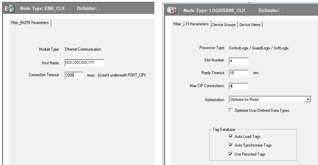
Figure 6-5 SMC ControlLogix PLC Configuration
