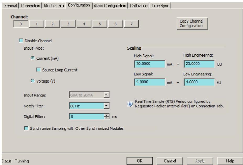
Figure 5-2 PLC Analog Input Card Range Configuration
