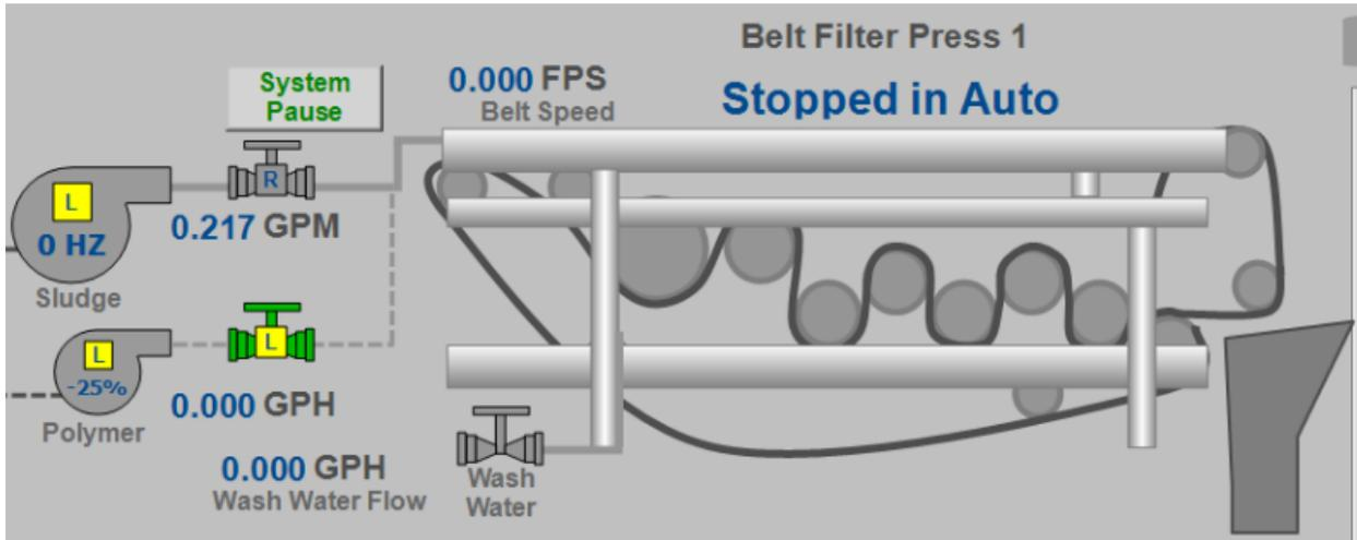
Figure 6-37 Belt Filter Press Graphic
