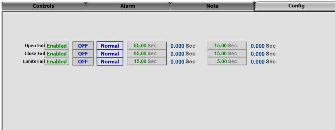
Figure 6-75 \$OpenCloseValves Template Popup Config Tab
