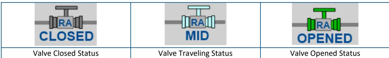
Figure 6-71 \$OpenClose Valves Template Graphic
