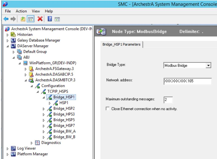
Figure 6-8 SMC Modbus Bridge Configuration
