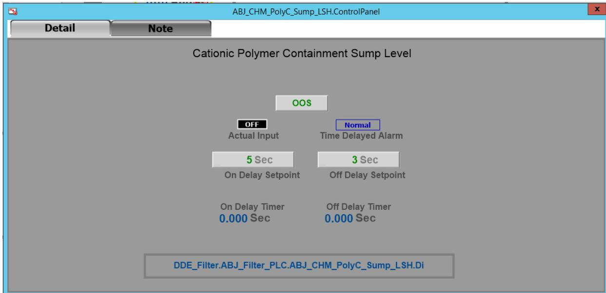
Figure 6-46 Discrete Alarm Popup Detail Tab
