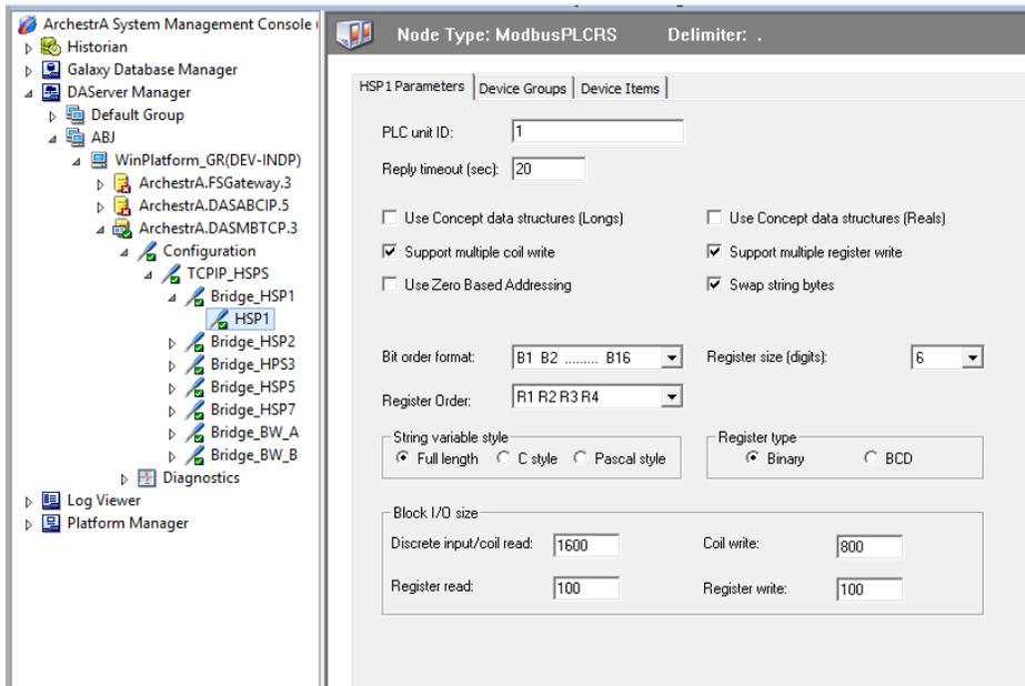
Figure 6-9 SMC Modbus Device Configuration for HSP Temperature Device
