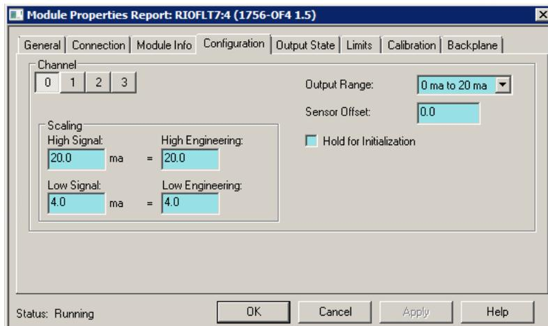
**Figure 5-4 PLC Analog Output Card Range Configuration**
