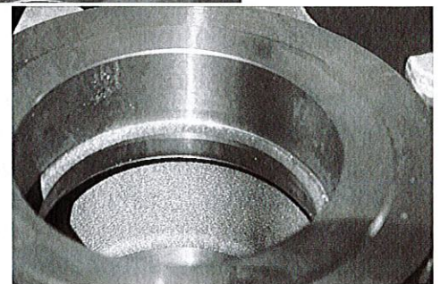
A 316L stainless steel machine welded seat ensures no leak through under the seat as you will often see when the seat is pressed in. The machined finish also gives precision so the resilient seat on the disc stops all media from flowing.
