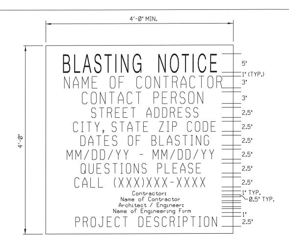
NOTE: SIGN TO BE CONSTRUCTED FROM 4'X 8'X 1/2" EXTERIOR PLYWOOD AND MOUNTED ON THE BACK BY 4"X 4" WOOD FENCE POSTS.
