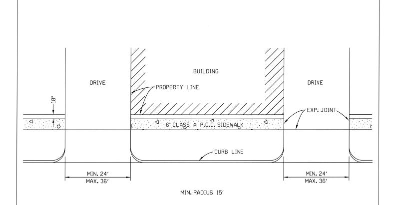
NOTE: CONSTRUCTION SHALL BE IN ACCORDANCE WITH STANDARDS 701 THROUGH 704 EXCEPT THAT COMMERCIAL DRIVES INCLUDING SIDEWALKS IN DRIVE AREAS SHALL BE A MINIMUM OF 6" THICK, CLASS A P.C.C.
