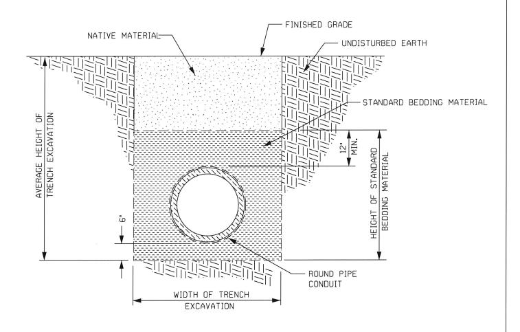
LIMITS OF STANDARD BEDDING MATERIAL QUANTITIES FOR BEDDING MATERIAL DO NOT INCLUDE THE SPACE WITHIN AND BOUNDED BY THE OUTER SURFACE OF THE PIPE CONDUIT.
