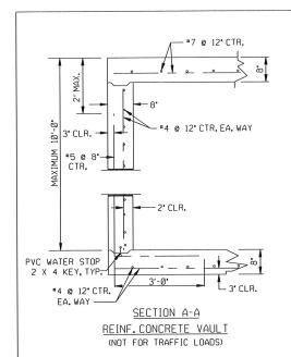
15" LIFTING HOOK TYP. 4 REQ.--30'X 48'HINGED DOUBLE LID, NEENAH R-6663'NH, FRAME TO BE CAST IRON LID TO BE ALUMINUM OFF-STREET, ROOF SLAB PLAN, ONE PIECE LID TO BE CAST IRON IN TRAFFIC.
