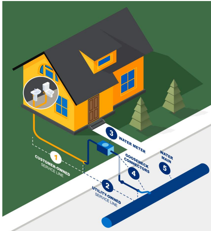
Figure 1. Water meter and service line orientation for City of Tulsa
