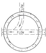
WHEN INSTALLING HYDRAULIC SLIDE THAT INTERCEPTS AN EXISTING SEWER AT A RIGHT ANGLE, THE CONNECTING INVERT OF THE HYDRAULIC SLIDE IS TO INTERCEPT THE EXISTING SEWER SLIGHTLY ABOVE THE SPRINGLINE AS SHOWN. DISTANCE MEASURED FROM INVERT TO INVERT.
