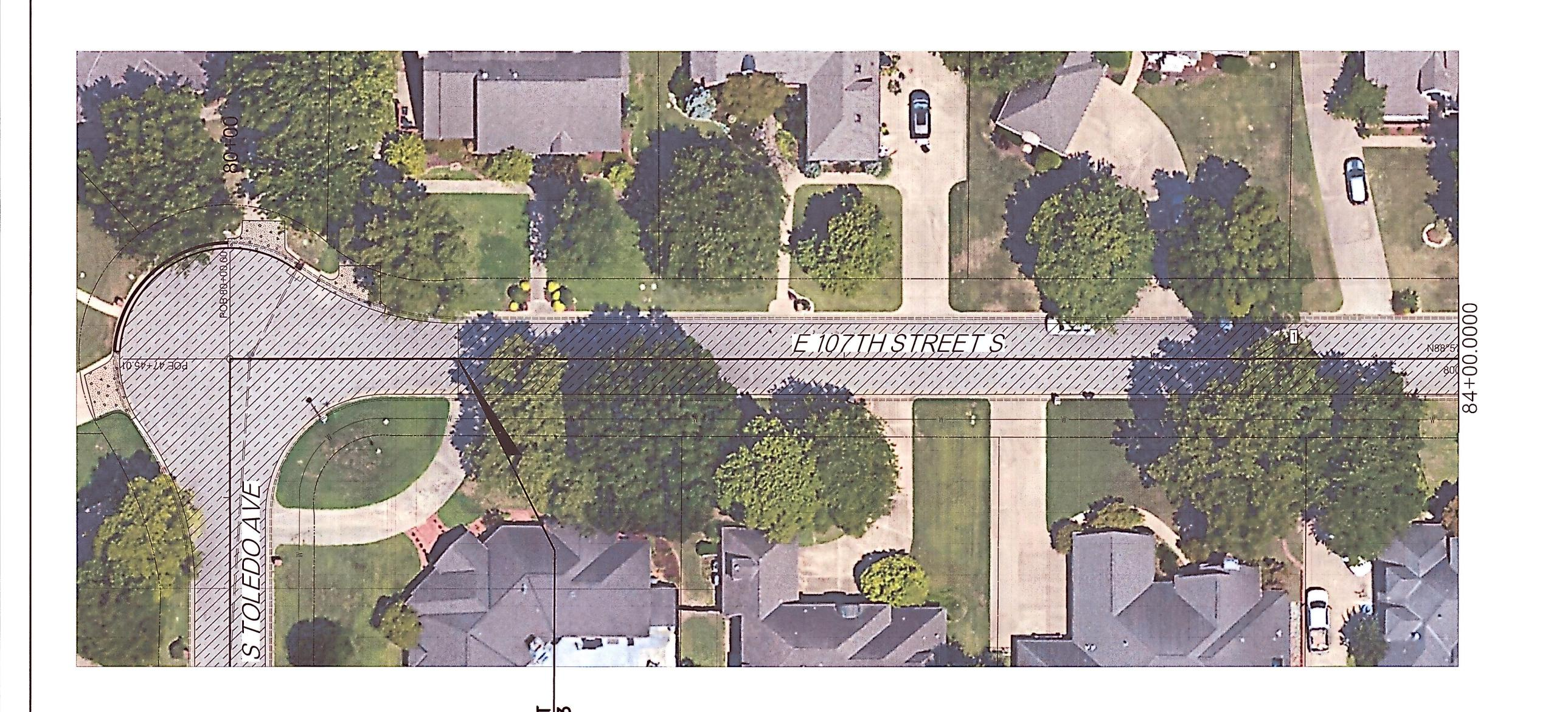
(VERT)1 inch = 5' ft. EGEND MANHOLE ADJUSTED TO GRADE VALVE BOX ADJUSTED TO GRADE CONSTRUCT CURB AND GUTTER CONSTRUCT CONCRETE DRIVEWAY MILL AND OVERLAY 6" CONCRETE DRIVEWAY
