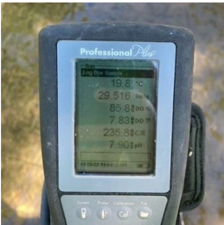
Figure 2: YSI multi-meter displaying pH, temperature, dissolved oxygen, and conductivity..
