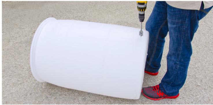
Drill two holes with a 1 3/16" or 1 1/4" drill bit, one toward the top of the barrel for an overflow and one toward the bottom of the barrel for the faucet.
