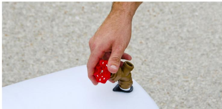
Twist in the threaded end of the faucet into the 3/4" threaded hole of the rubber gasket toward the bottom of the barrel.
