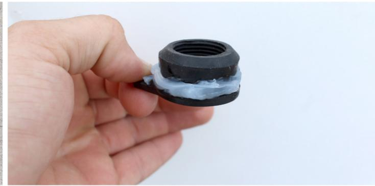
Prepare the smooth side of the 3/4" threaded rubber gasket with a bead of silicone caulk.
