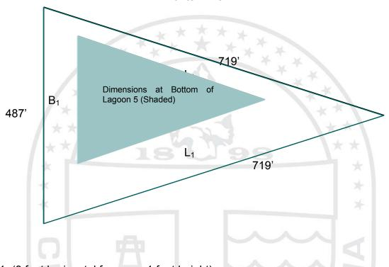
Slope is 3:1 (3 feet horizontal for every 1 foot height) Top dimensions at elevation 575.6.
