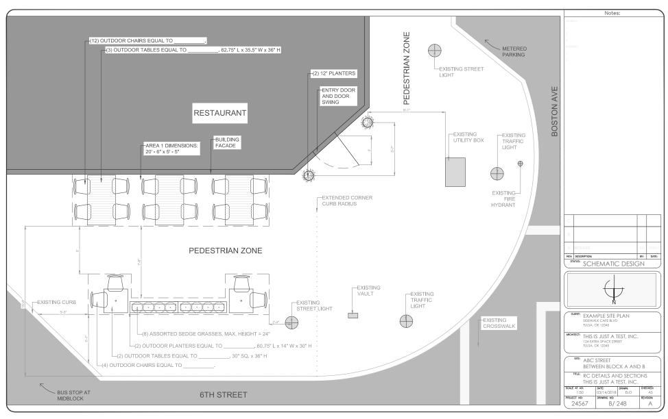
Note: This is only a graphic example of a site plan. Dimension requirements are subject to change. Both computer-aided site plan drawings and handdrawn site plans are acceptable. For handdrawn site plans, a Site Plan Graph Paper Template can be provided by the City of Tulsa. All drawings should be drawn to scale. All other site plan requirements can be found within this permit program manual.
